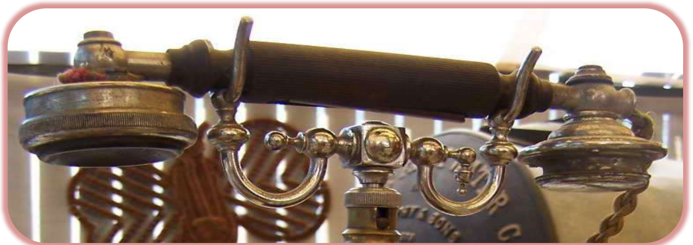
Cradle is missing one Teardrop
